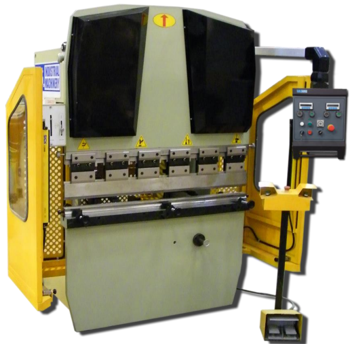
Photos above are manual Hydraulic Press Brake with front-operated power backgauge, power ram adjustment, both with manual fine adjustment and digital readouts. Operator's pendant has dwell adjustment for ram, key lockout, jog control and E-stop.
